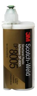
3M™ Scotch-Weld™ Structural Plastic Adhesive DP8005 is a 10:1 ratio, two-part, acrylic-based adhesive specially formulated to bond many low surface energy plastics. It will adhere many grades of polypropylene, polyethylene, and thermoplastic elastomers (TPEs) without special surface preparation.
